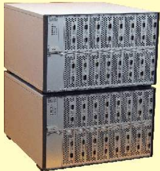
Two Cell Test Systems with together 64 independent test channels, each with 5V/5A.
