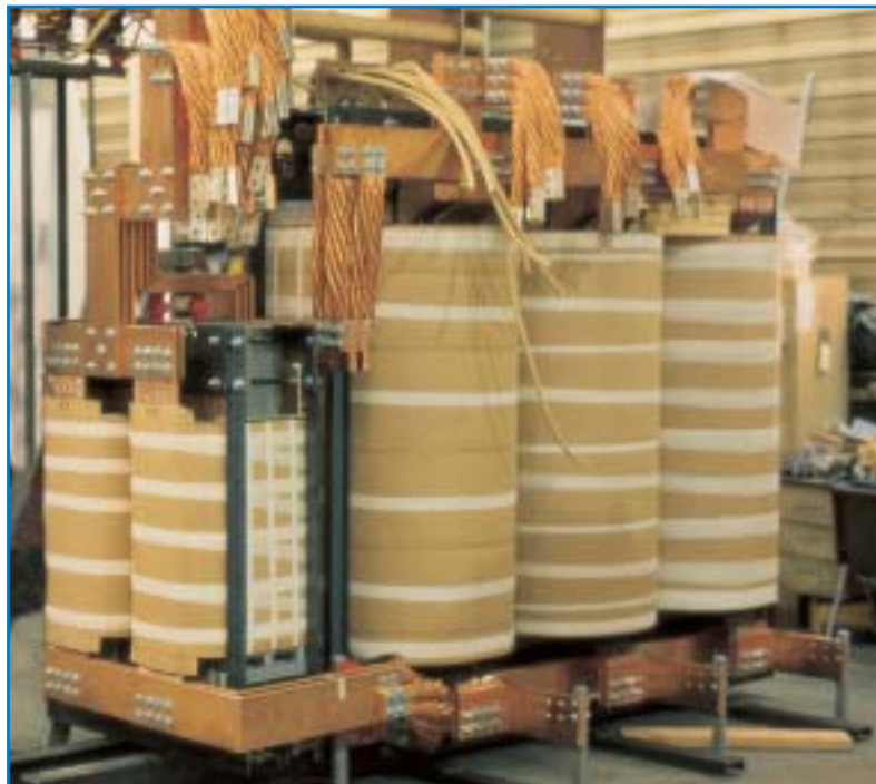
Core and coil being tested prior to final assembly
