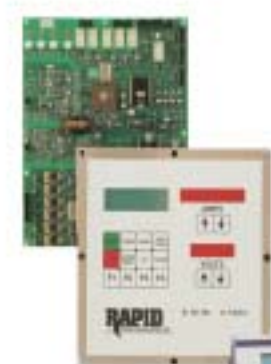
Basic digital controller and HMI panel
