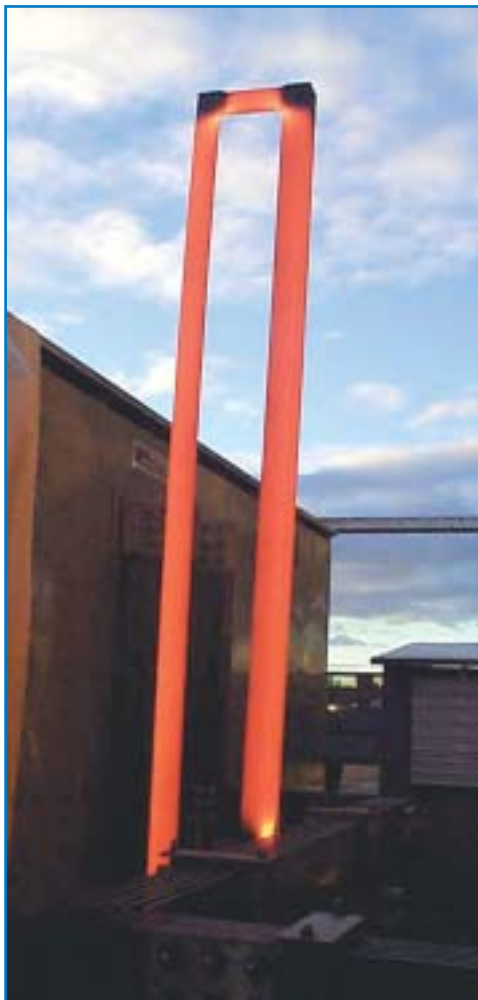
Field testing a high power rectifier with substitute load
